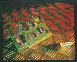
If desk space is starting to get a bit tight and you're lucky enough to own an Amiga capable of handling Zorro cards (an A2000 or A4000, for example), then you may well want to check out the Supra 2400zi. This is more suitable for A1500 owners because it fits internally. It has a maximum transfer speed of 2400 baud but doesn't offer error correction or compression.
