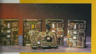
**IDE stands for Intelligent Drive Electronics** and SCSI stands for Small Computer System Interface. IDE drives are currently to be found inside the A4000-40, the A4000-30, the A600 and the A1200. At present SCSI drives are in the A1500, 2000, 3000, 500, 500 Plus.
