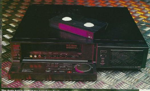
The Sony 517 is perfect for a post production video editing set-up. It has all the features you'll need including a tight frame freeze, jog and shuttle, LANC sockets and plenty of input ports.
