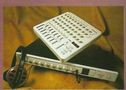
The Fostex rack-mountable DCM100 line mixer offers eight stereo channels.
